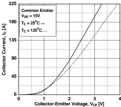
Figure 4. Transfer Characteristics
