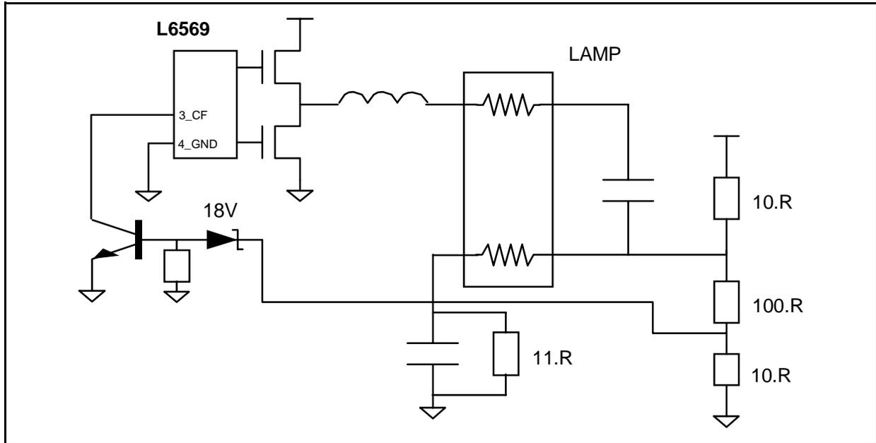
Several ways can achieve the protection task. First it can be done by sensing the resonant current through a MOSFET source resistor or a secondary winding on the choke. The switching is stopped when a large current reduction is detected by analog means.
