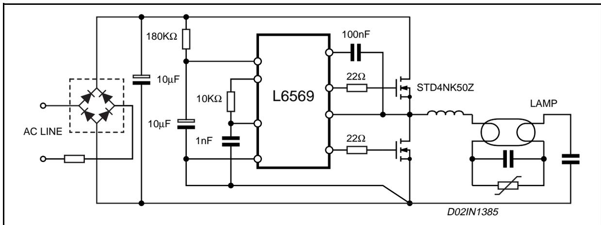
Figure 5: Bootstrap capacitor charge.
