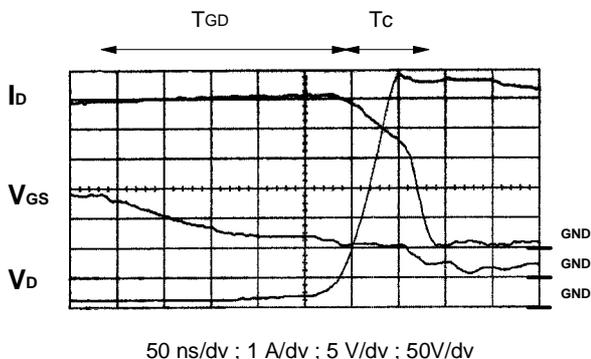
The built-in dead time circuit acts when a MOSFET turns off, delaying the turn on of the opposite transistor for  $1.25 \mu\text{s}$ . The voltage  $V_{OUT}$  between the 2 MOSFETs must switch within the minimum dead time ( $0.85 \mu\text{s}$ ), as shown on figure 8, to avoid bridge cross conductions and transistors overheat.
