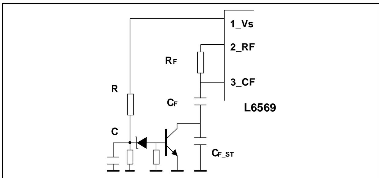
line voltage  $V_{DC}$  is applied when the oscillator starts. The ballast has to start directly with its nominal conditions to remove any transient oscillation. Hence the operation runs in ZVS mode with no spurious lamp ignition. This situation does not occur with the saturable transformer drive, because the saturation limits naturally the current by increasing the frequency.
