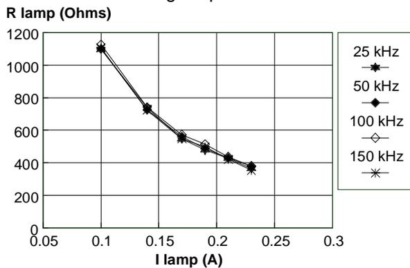
From the tests the impedance appears insensitive to the frequency for such lamps. The specified impedance might be valid for higher frequency operation. The relative lamp light output was measured as proposed in reference [5]. The light flux increases slightly in that frequency range, but can be considered constant.
