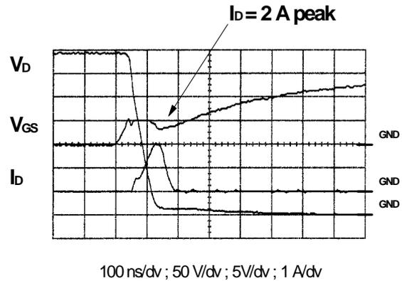
**Figure 22:** Open load detection example.
