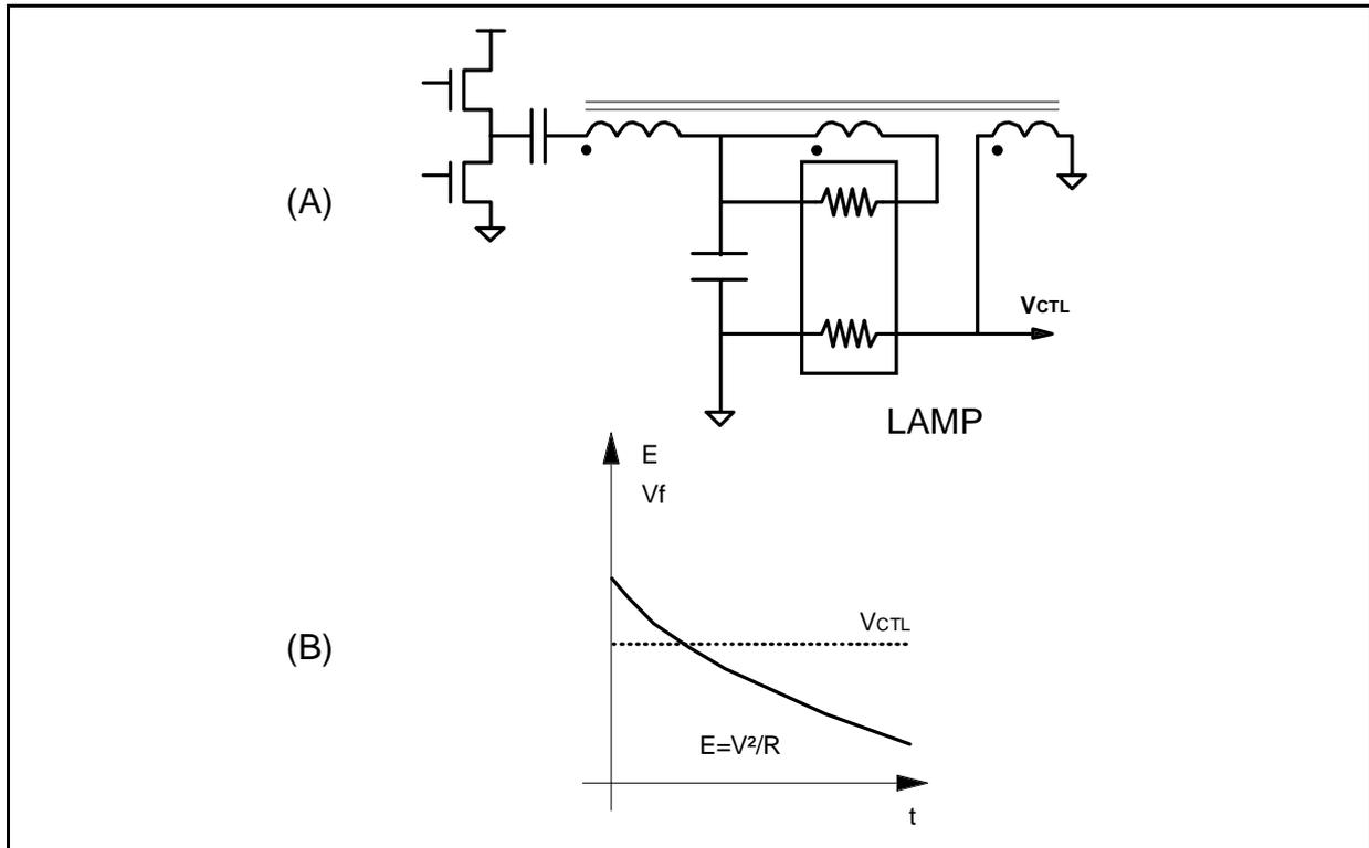
**Figure 18:** Double frequency control for the L6569 with programmed frequency and duration.
