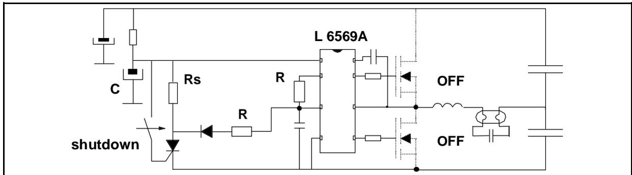
**Figure 13:** L6569 disable circuitry with both MOSFETs off.
