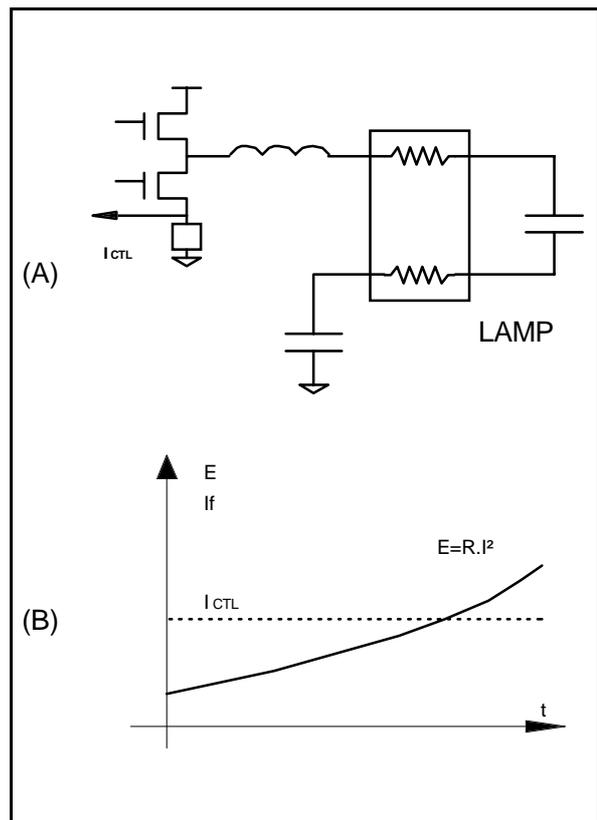
The preheat can be achieved with a filament voltage control. The filaments are supplied by two auxiliary windings of the resonant choke as shown figure 17a. During the preheat the L6569 frequency is increased, and the choke operates
