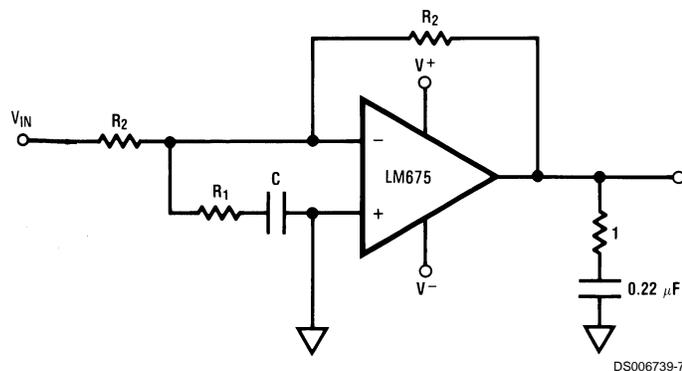
$$R_1 C \geq \frac{1}{2\pi 500 \text{ kHz}}$$
