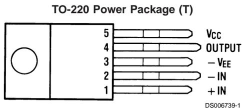
\*The tab is internally connected to pin 3 ( $-V_{EE}$ )
