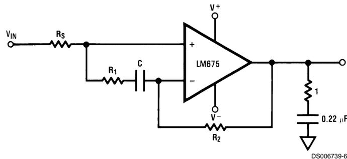
$$R_1 C \geq \frac{1}{2\pi 500 \text{ kHz}}$$
