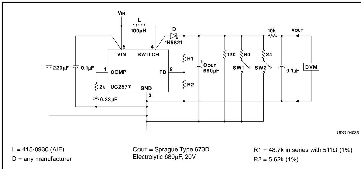
Figure 1. Circuit Used to Specify System Parameters
