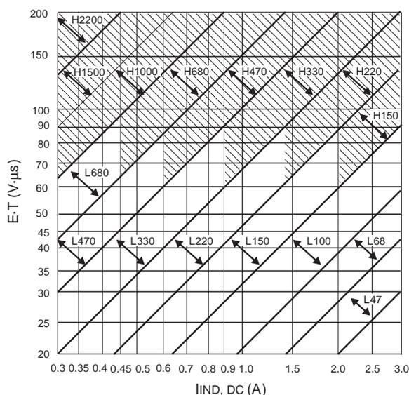
Note: This chart assumes that the inductor ripple current is approximately 20% to 30% of the average inductor current (when the regulator is under full load). Greater ripple current causes higher peak switch currents and greater output ripple voltage. Lower ripple current is achieved with larger value inductors. The factor of 20% to 30% is chosen as a convenient balance between the two extremes.
